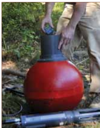
A researcher places a MoteStack monitoring device into a buoy.
