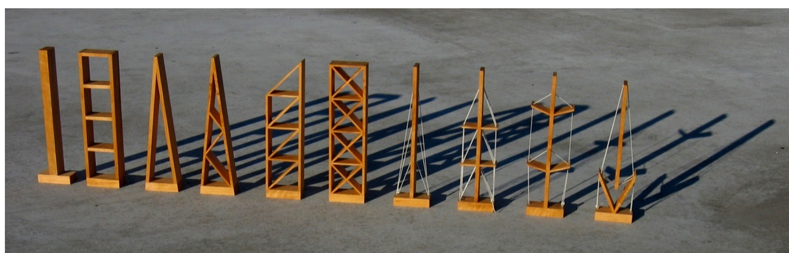
Point of origin: summary of loadbearing principles for vertical structures.
