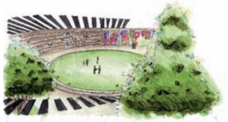
The amphitheater is a mounded lawn surrounded by raised stone seating. Rainwater harvesters surround the area creating a unique yet environmentally friendly area. Water harvested from these features will be used to meet the site's irrigation needs.
