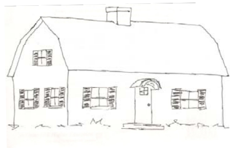
FIGURE 7.5 GAMBREL ROOF. DRAWING BY AUTHOR. 17 MAR. 2010.
