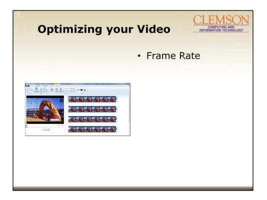
Frame/Rate – this is the actual number of frames per second at which you are currently recording. Average video camcorder captures motion at 30fps. Motion picture films are slower at 24 fps. Screen capture video ideally should be around 12 to 15 fps. If you are just recording a presentation like a PowerPoint 1 to 2 fps should be fine.
