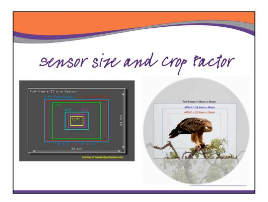
The crop factor is the sensor's diagonal size compared to a full-frame 35 mm sensor. It is called this because when using a 35 mm lens, it **crops out this much of the image** at its exterior (due to its limited size).
