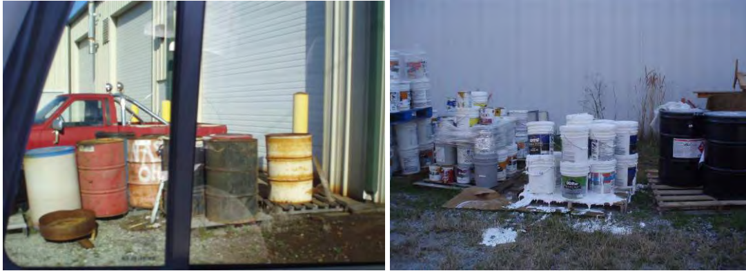
Figure 6.40. (a) Storage of 55 gallon drums at Plinkington Advanced Technologies (K-HSI-3) without cover or secondary containment and (b) leakage and spilling from paint containers at 1 Sunblet Ct. (K-HSI-4).
