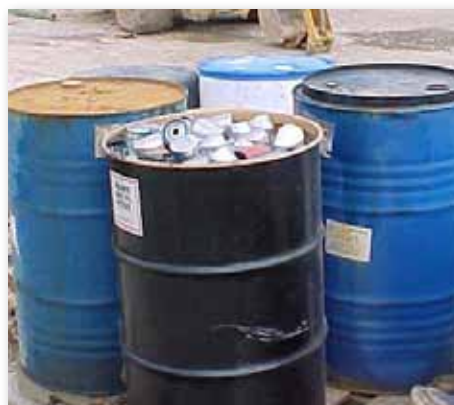
Used motor oil and oil filters incorrectly stored where rain can fall on them. Photo courtesy of Brian Wisnewski.
