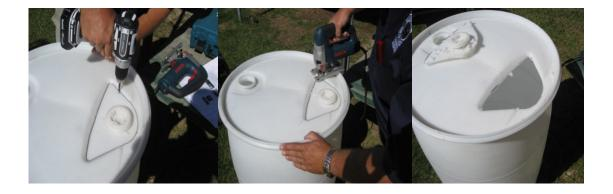
3. Drill a hole (with a 1¾" hole saw or 1¾" paddle bit) at the top of the barrel for an overflow and one at the bottom of the barrel for the spigot. If barrel will not be elevated locate hole for spigot high enough to attach hose without crimping.
