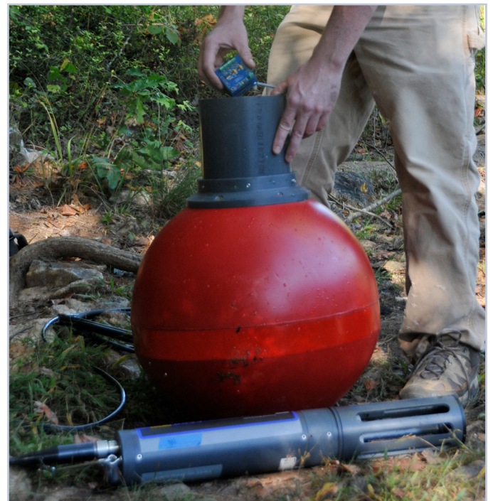
A researcher places a MoteStack monitoring device into a buoy.
