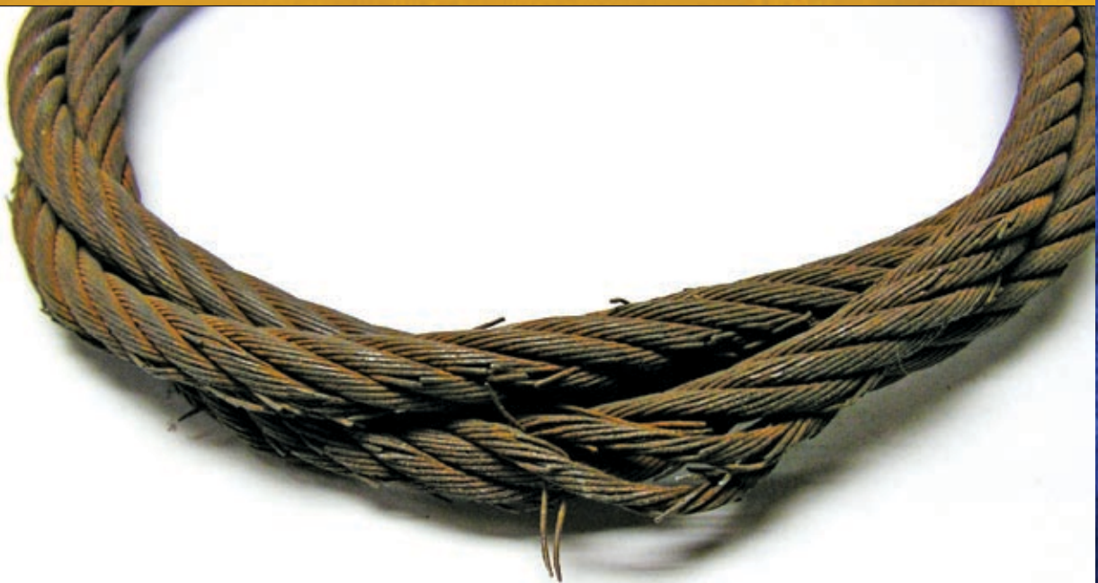
The anchor point is pulled out, making the whole web device ineffective. Broken individual wires (below) weaken the cable and create injury potential for persons handling it.
