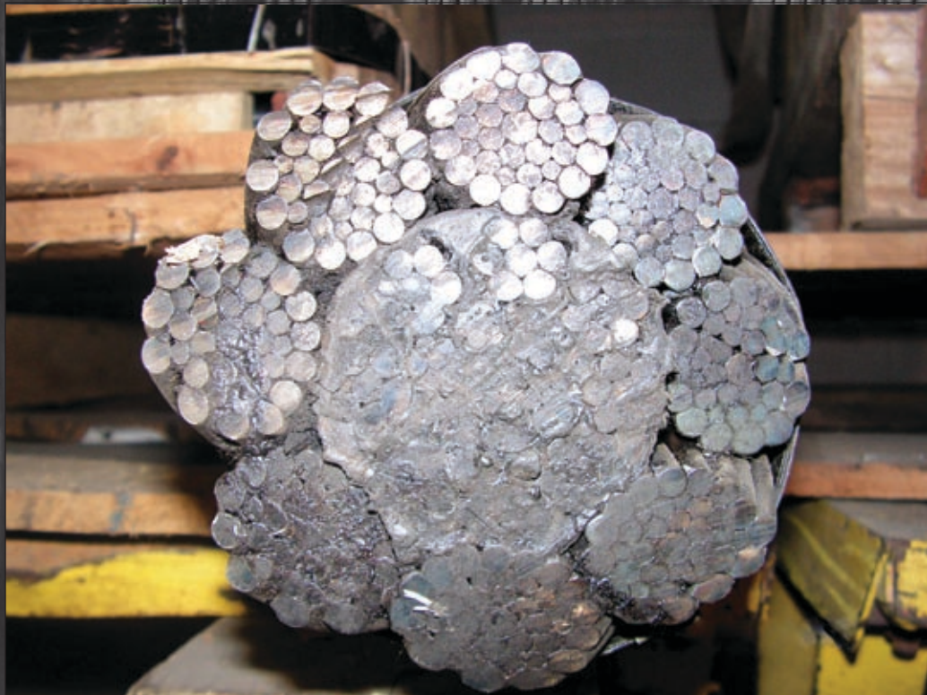
Wire ropes (above and below) showing center cores wrapped by individual bundles.
