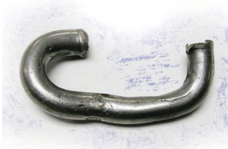
A chain link that broke at the weld when the pressure exceeded its breaking strength.
