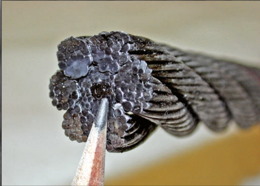
Wire ropes (above and below) showing center cores wrapped by individual bundles.
