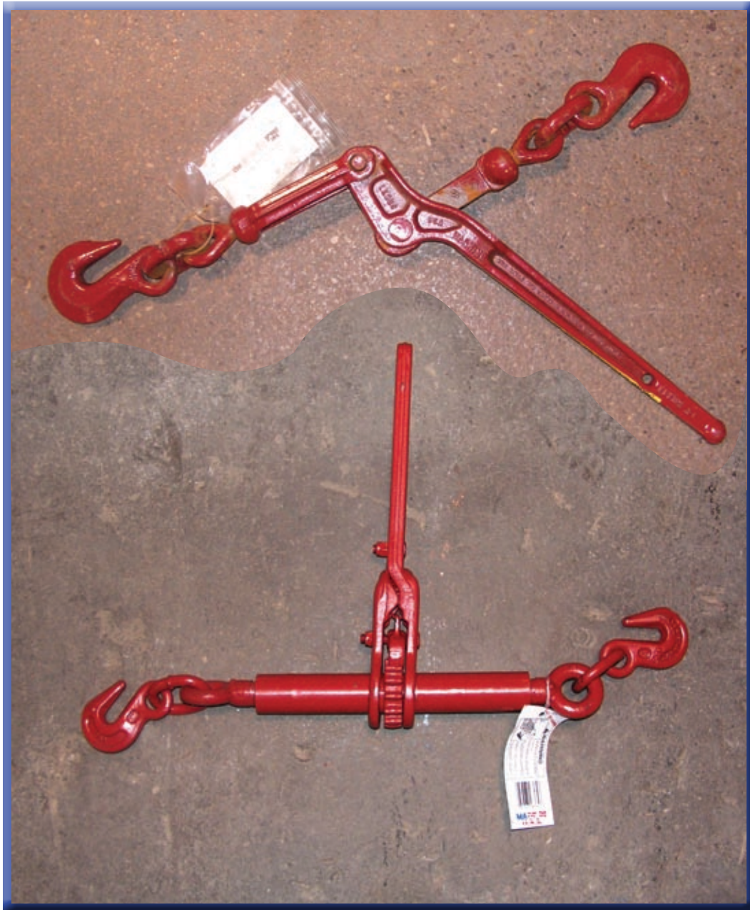
A pull-over-center binder (top) and a ratchet (bottom).
